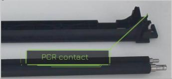
22. Clean the black conductive saddle with a cotton swab, then apply a small amount of conductive grease into it.
